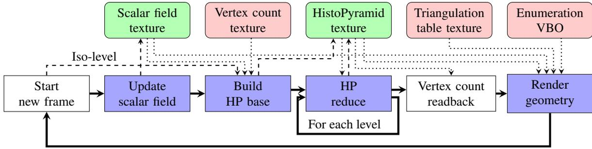
Figure 7: A schematic view of the implementation. Thick arrows designate control flow, with blue boxes executing on the GPU and white boxes on the CPU. The dotted and dashed arrows represent data flow, with dotted arrows for fetches and dashed arrows for writes. Green boxes stand for dynamic data. Red boxes for static data.
